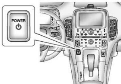
The vehicle has an electronic push-button start. The POWER
