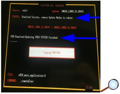
Important: Once the updating file hits 90% the screen may go blank, DO NOT REMOVE the USB at this time. The illustration above shows when the programming is complete. (See blue arrows above.)
